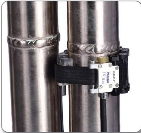
Bracelet scanning a 2" pipe (5mm W/T) with a single phased array probe
